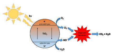
Figure 4: The mechanism of photocatalysis.
