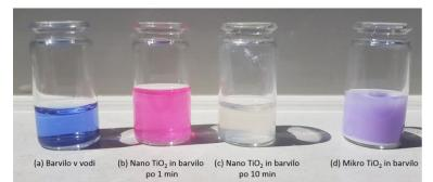
Figure 3: The reaction between the Resazurin dye and nano  $TiO_2$ . (a) Dye in water (b) Nano  $TiO_2$  and dye after 1 min (c) Nano  $TiO_2$  and dye after 10 min (d) Micro  $TiO_2$  and dye
