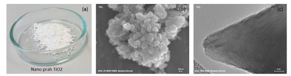
Figure 1:  $TiO_2$  nanopowder. (a)  $TiO_2$  as seen by the naked eye, (b) a cluster of  $TiO_2$  particles and (c) a single  $TiO_2$  particle as seen using electron microscopy.
