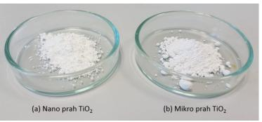
Figure 2: TiO<sub>2</sub> nanopowder and TiO<sub>2</sub> micropowder.
