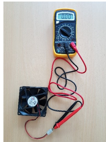
Figure 5: Voltage measurements with a multimeter
