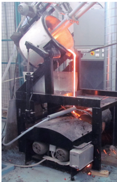
Preparation of mineral fibres for heat insulation applications: Fiberization of the melt on two-wheel spinner with frequency controller.
