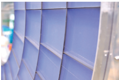
The Cherenkov radiation occurs in the transmission of charged particles with the velocity higher than the speed of light through the silicon aerogel plate into the matter.
