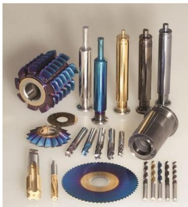
A Slovenian public research organization has developed several types of hard protective coatings to increase the lifetime of tools in machining. The benefit of deposited coatings is in their improved mechanical properties such as hardness, chemical inertness and adhesion. Partners that wish to prolong the lifetime of cutting and forming tools are sought for commercial agreements with technical assistance.
