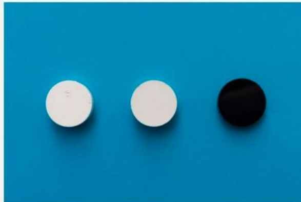
Figure 2. Photograph of nanocellulose-zirconia before (left) and after (right) SPS – spark plasma sintering. After sintering it turns black due to graphitization of the nanocellulose. The black sample is highly electroconductive (400 S/m).
