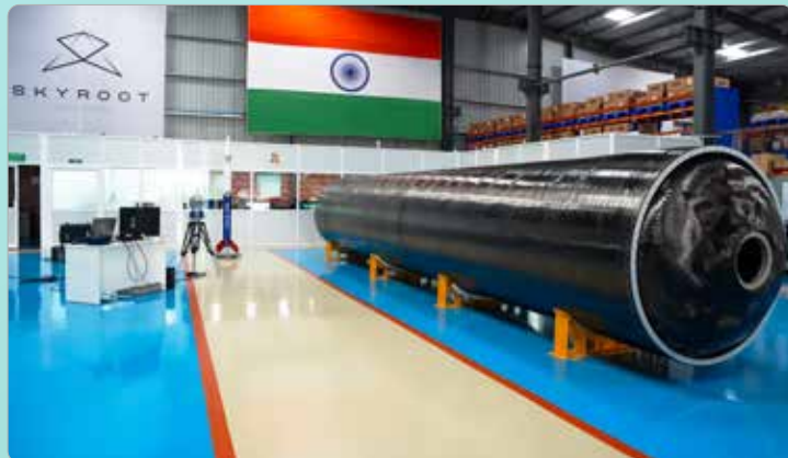
Vikram-1 Stage-1 Kalam 1200 Solid Rocket Motor Case
