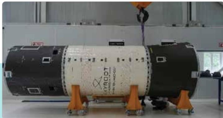
Carbon Composite Interstage Structures
