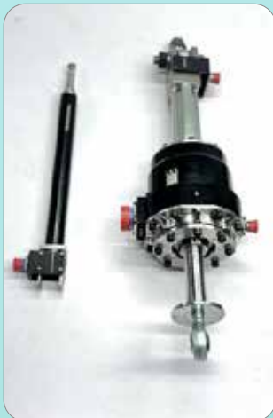
Thrust Vector Control System (Actuator, MI Sensor)
