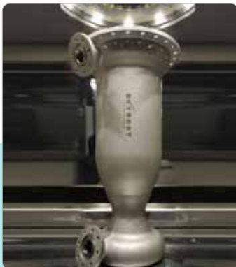
3D-Printed Dhawan-I Cryogenic Engine
