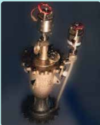
3D-Printed Raman-II Liquid Propulsion Engine
