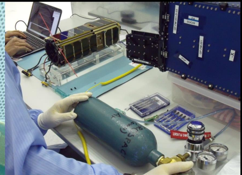
14 Dec 2014 11:28 SGT - Firing P 1.62bar DC 90% axis -Y 10sec x 4 followed by axis +Y 10sec x 3
